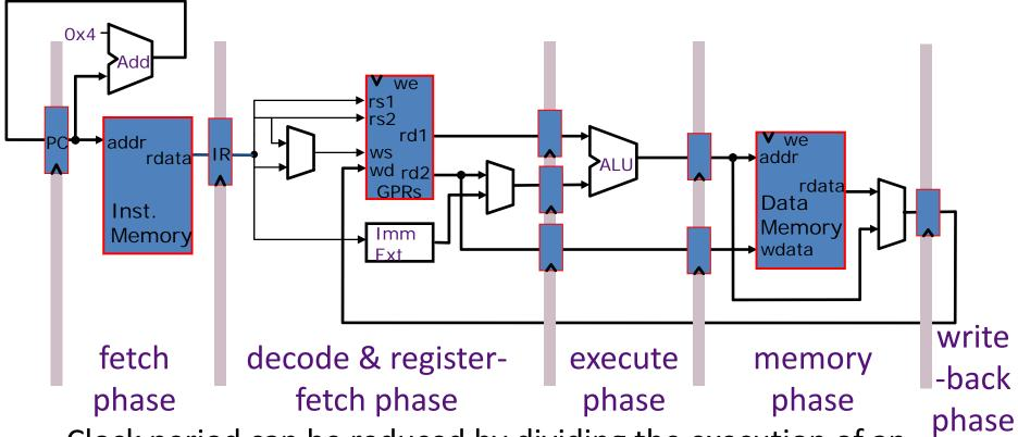
Clock period can be reduced by dividing the execution of an instruction into multiple cycles
