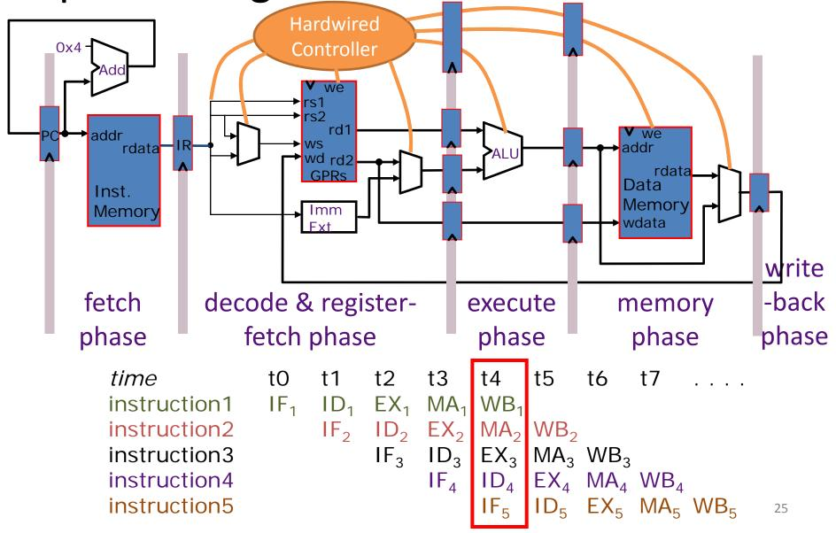
Pipeline Diagrams: Space vs. Time
