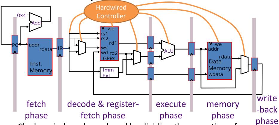
Clock period can be reduced by dividing the execution of an instruction into multiple cycles
