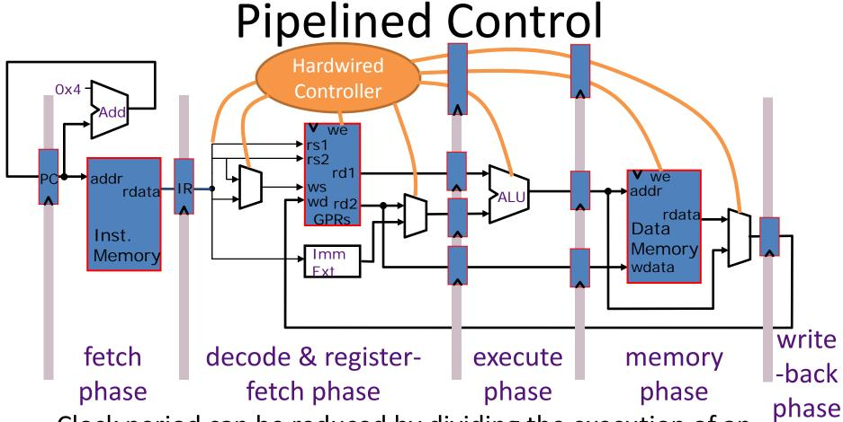
Clock period can be reduced by dividing the execution of an instruction into multiple cycles
